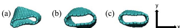
Figure 5. Snapshot of the CNT at its maximum deformation. Drawn in (a), (b), and (c) are the CNTs interacting with PS, poly(DMAEMA), and poly(DMAEMA-co-St), respectively. The CNT lies along the Z-axis and polymers are not shown. Drawn in cyan, blue, and red are carbon, nitrogen, and oxygen atoms, respectively.
